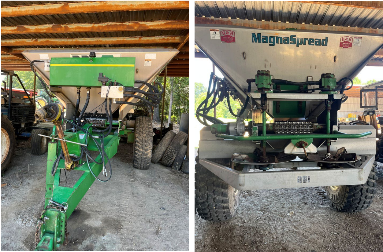
Figure 3. BBI MagnaSpread spreader used for CarbonLock spreading. Left: control and hydraulic systems. Right: conveyer belt and spinning disks throw CarbonLock off the back of the spreader. This is fed by the large hopper on top.
