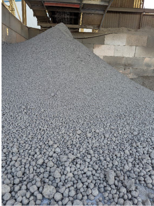
Figure A2-4. O.C.O manufactured limestone (M-LS) aggregate product after pelletizing.
