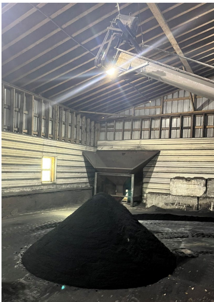
Figure 2. Biochar dispensed into staging room from screw auger.
