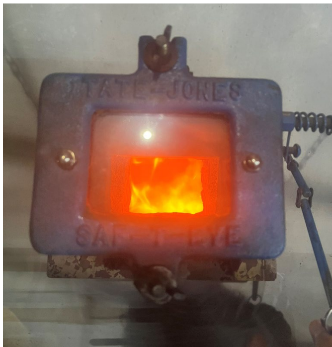
Figure A2-3. Inspection port on lower stage of gasifier.
