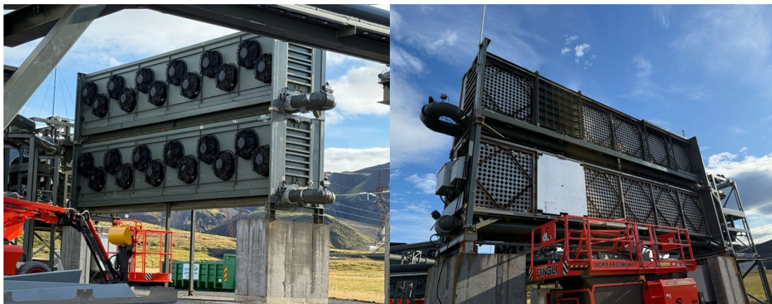
Figure 2: Left. Rear of contactor containers showing array of fans for drawing CO 2 across sorbent material. Right. Isolation door of contactor container sub-units for application of heat and vacuum for CO 2 desorption.
