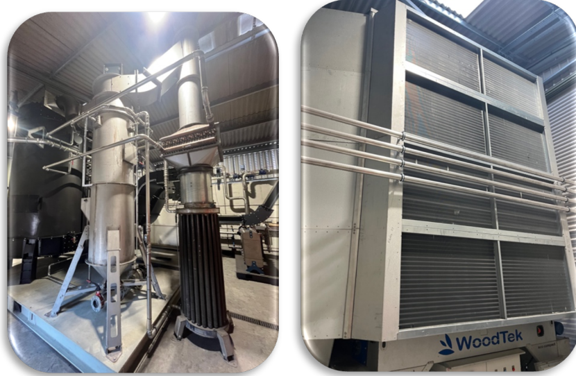
Figure 4: C-1000 pyrolysis technology showing the two biochar outfeeds, the scrubber and dryer installed at the facility
