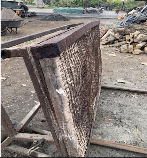
The door made to improve and speed up warming
