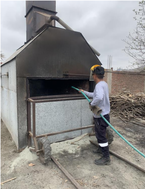
Cooling the charge with a water hose to advance the test.
