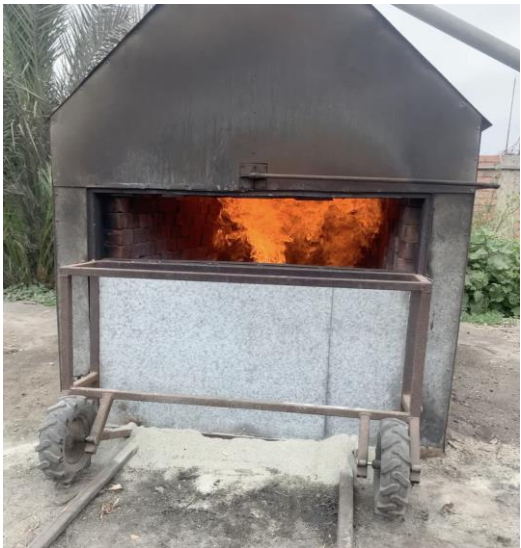
The bottom of the reactor is sealed with grave
