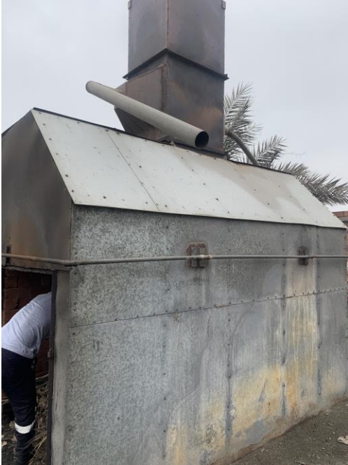
Reactor from the top a hot air outlet pipe
