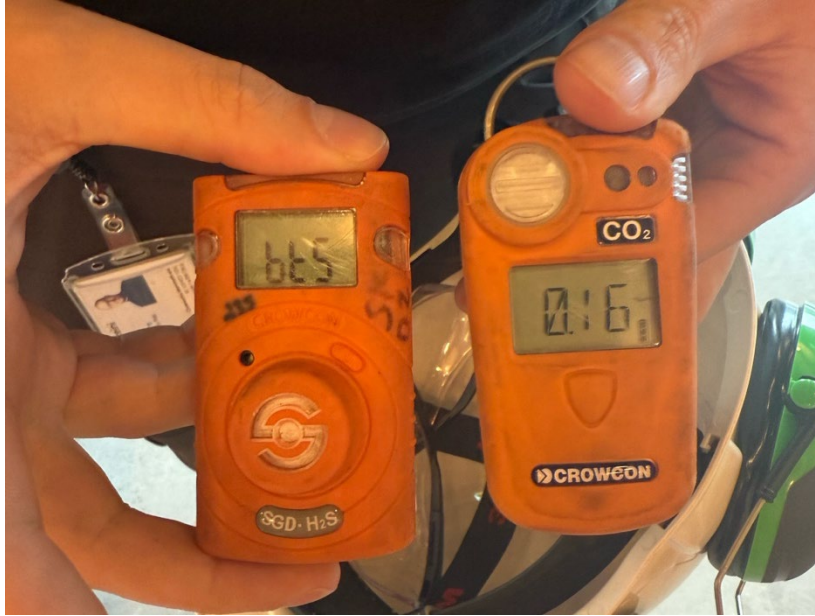
Figure A: CO 2 and H 2 S sensors used by Climeworks staff as part of their HSE equipment
