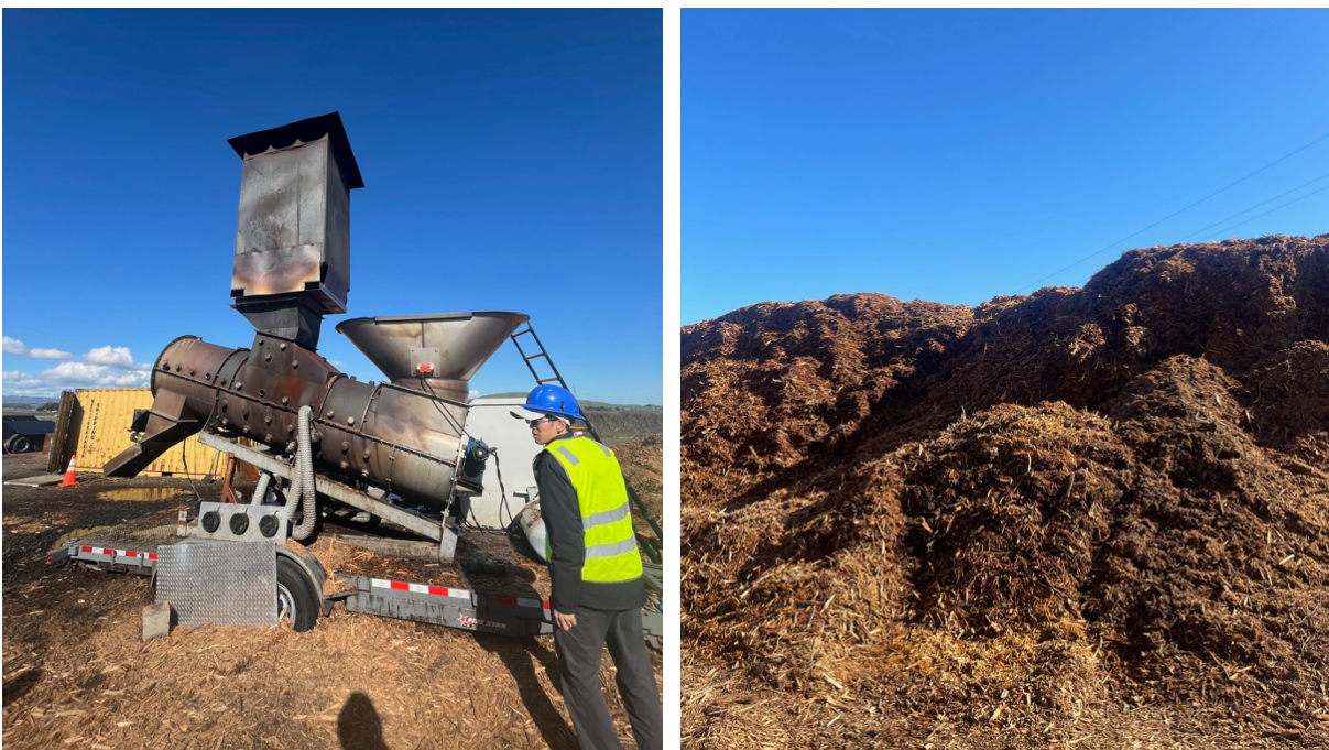
FIGURE 1 DOUGLAS BIOCHAR REACTOR (LEFT), BIOMASS PILE DUMPED ON SITE BY TREE MANAGEMENT CONTRACTORS (RIGHT)
